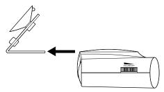
To adjust the mounting angle, remove the detector from the bracket. Then, remove the bracket from the windshield and adjust it by carefully bending it.
